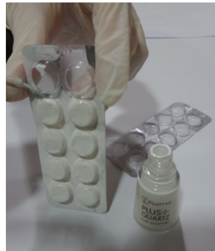
Figure 2: The boundary and bottom coated by white nail paint
