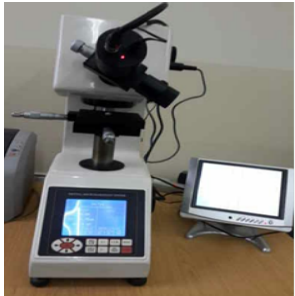
Figure 7: Digital microhardness tester
